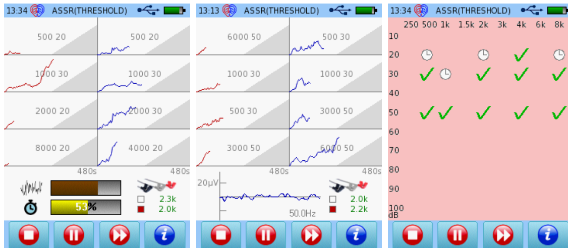
Fig. 31: Representation of ongoing test: Left: Default view, representing the 8 ASSR channels; mid: alternative view with raw EEG; right: status view for right ear, indicating finished and ongoing points
