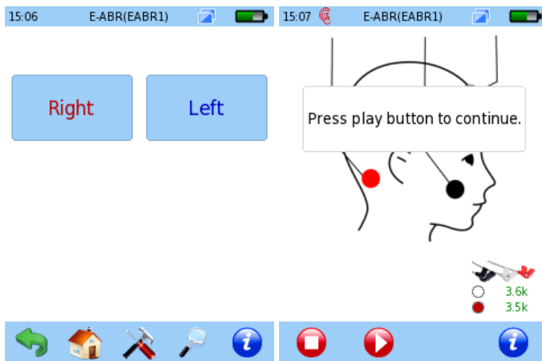
Figure 6: Ear selection (left) and impedance pre-check (right) on the SENTIERO ADVANCED
