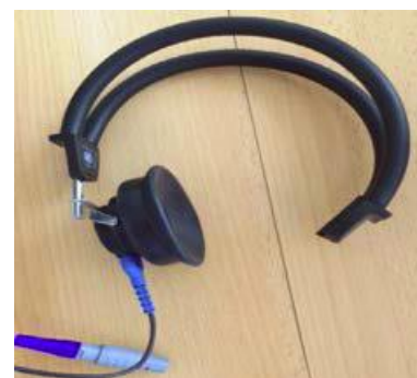
Figure 1 From Left to Right: a) VIP Probe, b) Binaural DD45 headphones, c) Monaural DD45 option
