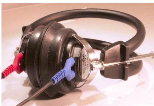
Figure 1 From Left to Right: a) VIP Probe, b) Binaural DD45 headphones, c) Monaural DD45 option
