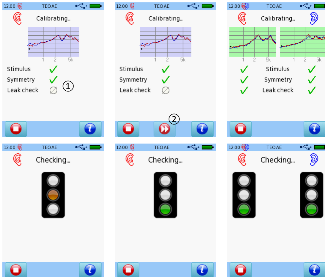
Figure 32: TEOAE ear probe calibration (top left: expert mode monaural; top middle: expert mode monaural with skip option; top right: expert mode binaural; bottom left/middle: simple mode monaural; bottom right: simple mode binaural)
