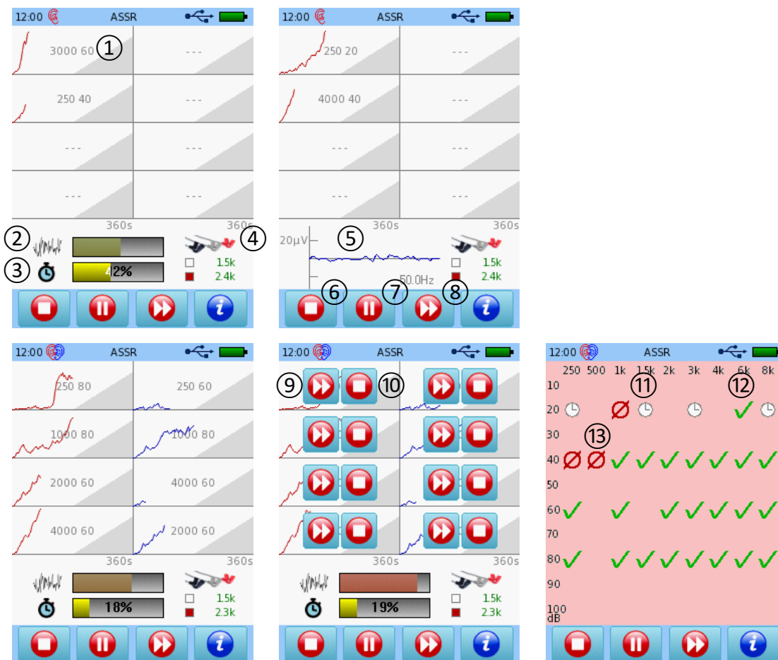
Figure 62: ASSR measurement (top: monaural 40 Hz ASSR measurement; top left: standard measurement screen; top right: measurement screen with EEG noise graph; bottom: binaural 80 Hz ASSR measurement; bottom left: standard measurement screen; bottom middle: skip/stop selection; bottom right: measurement status and result matrix)
