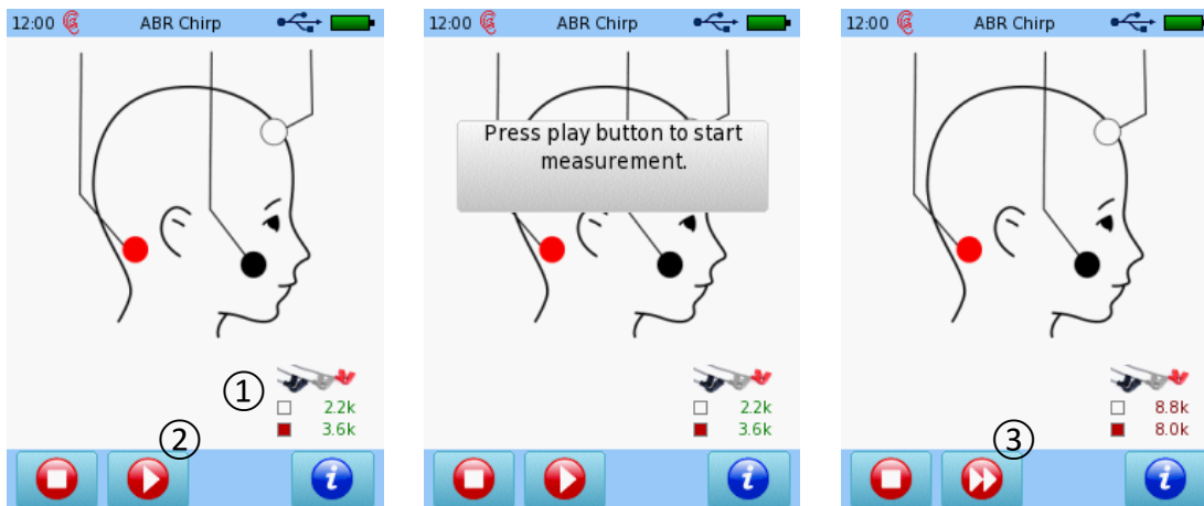
Figure 49: ABR impedance measurement (left: good impedances with play button; middle: good impedances with play button and reminder to start test by pressing the play button; right: poor impedances with forward button)
