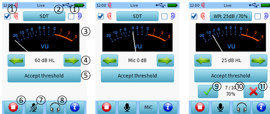
Figure 22: Live Speech user interface (left: SDT user interface with microphone turned off; middle: SDT user interface with microphone turned on and microphone level adjustment; right: WR user interface after accepting the determined threshold)
