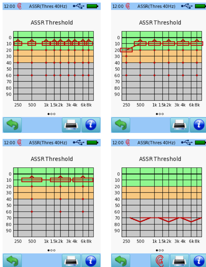
Figure 64: ASSR Threshold result (top left: 1/2 octave stimulus bandwidth; top right: octave stimulus bandwidth; bottom: two octaves stimulus bandwidth).
